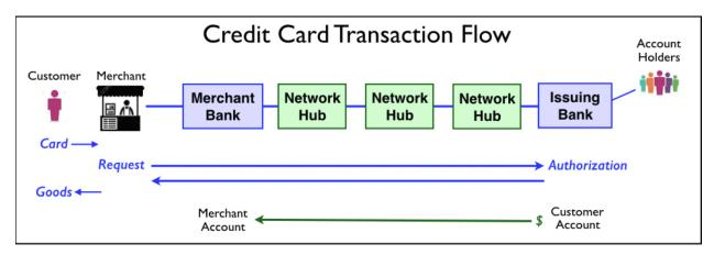
A customer inserts his card into a POS device at a merchant. A request is sent from the merchant through the card infrastructure to the customer's issuing bank, which authorizes the transaction and sends a response back to the merchant. At a later time, funds follow the transaction trail, from the customer's account to the merchant's account.
